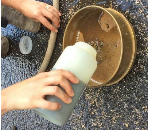
Sediment samples were poured into a mesh sieve in order to filter out small particles
