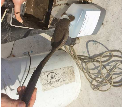
Sediment samples were transferred into a Nalgene bottle in order to transport sediment samples to Aquatic Systems, where larval counting took place
