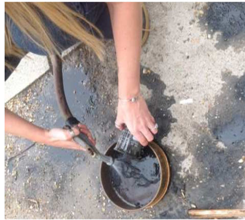
Small particles were washed through the mesh sieve
